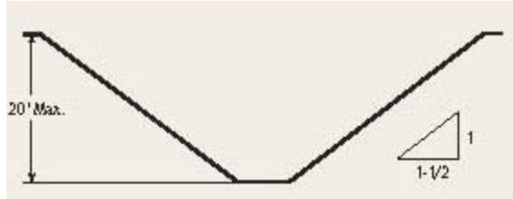
Figure 1. Excavations Made in Type C Soil
